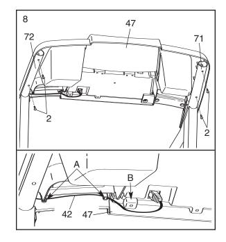
Cover the Upright Wire (42) with the Right Grip Plate (36). Be careful not to pinch the Upright Wire. Tighten two 1/2" Screws (48) and the 3/4" Screw (2) into the Right Grip Plate and the Console Base (47).
